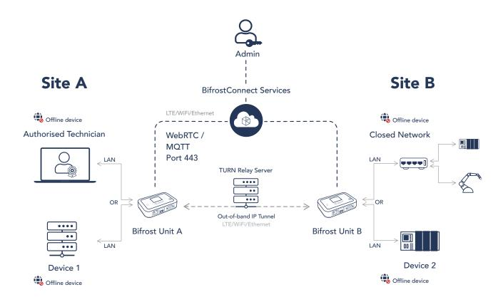
The Bifrost IP Tunnel is designed to provide a secure end-to-end encrypted connection between two Bifrost Units. These Point-to-Point tunnels are created on a per-session, on-demand basis, and all session data is transitory and will not be stored on any server.
