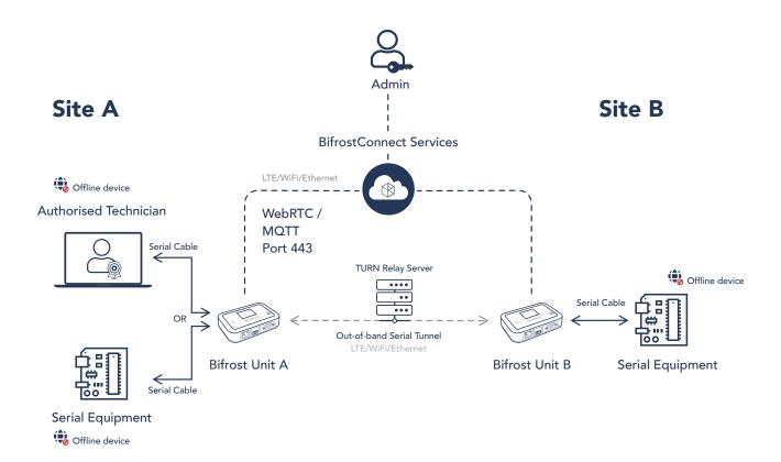
A Bifrost Serial Tunnel facilitates a secure, encrypted session between two Bifrost Units. These tunnel sessions are initiated just in time, safeguarding sensitive information by ensuring session data is transient and never stored on servers.
