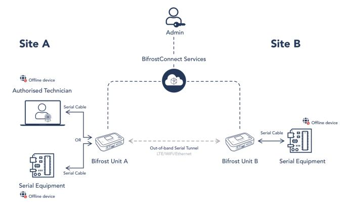
Bifrost-to-Bifrost Tunnels 2: Serial Tunnel
