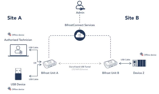
Bifrost-to-Bifrost Tunnels 3: USB Tunnel
