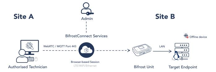
KVM & Console Setup 3: SSH Sessions facilitate the transmission of keyboard strokes (no file transfer) to the console's terminal.
