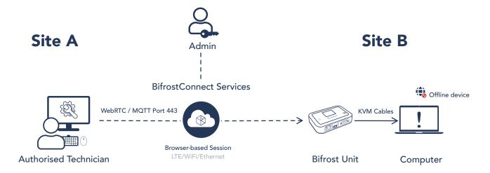
KVM & Console Setup 1: KVM Access Sessions facilitate the transmission of keyboard, video, and mouse (KVM) I/O signals.
