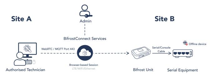
KVM & Console Setup 2: Serial Terminal Sessions facilitate the transmission of keyboard strokes to the console's terminal.
