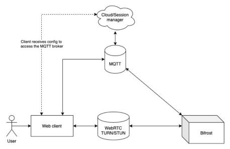
In the BifrostConnect solution, both the web client and the Bifrost Unit authenticate themselves to the BifrostConnect Service, communicating over industry-standard encrypted channels utilizing Transport Layer Security (TLS). This encryption is separate from the peer-to-peer (P2P) encryption that occurs between the web client and the Bifrost Unit, which is secured via Datagram Transport Layer Security (DTLS) encryption through WebRTC.
